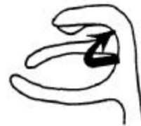
Fig. 10-6.■ The angle between the rest and the proximal minor connector is less than 90 degrees
